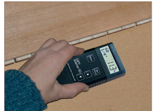
Correction for domestic and tropical wood species, panel products and subfloors. Can be self-calibrated for engineered products.
