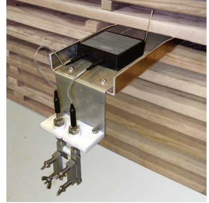
EMC measuring station with transmitter sends EMC measurements directly to receiver to keep track of ambient conditions and climate in a dry kiln.
