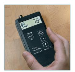
Pinless mode: fast and easy moisture checking of lumber and flat boards.
