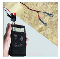
Install cables and pins in moisture critical areas.
