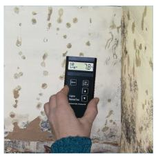
Ligno-VersaTec has a true percent scale for drywall and reference scales to evaluate moisture conditions in other building materials.
