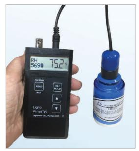
The HR75 bottle lists temperatures and the corresponding relative humidity values. Check for a maximum variation of +/-2% from your measurements for ASTM F2170 concrete testing. Values for 75% are listed balow. For values for 33% at different temperatures, check the salt bottle.
