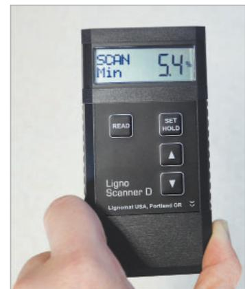
**Step 2:** Closed circuit check. Place the pinless meter on your forearm and press the READ key. A high moisture value should be indicated. An additional meter check can be performed by measuring a ream of paper. If the paper test is done repeatedly with the same setting, the indicated value should not vary significantly over the course of a year. This can be used to check consistency / accuracy of the pinless calibration.
