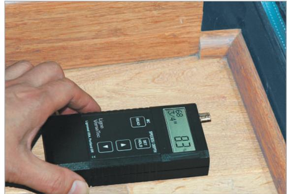
**First:** Take measurements when the floor is delivered, to make sure the floor is dry.
