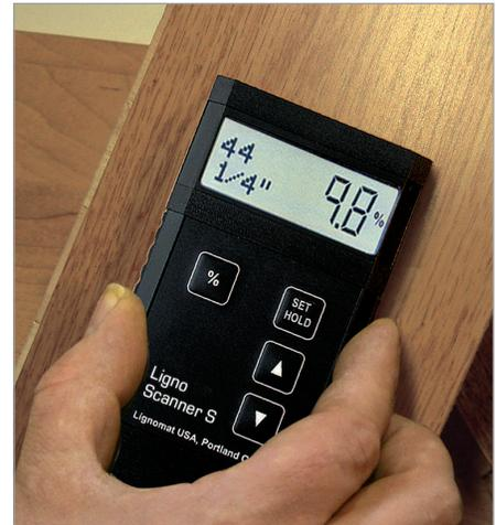
All Lignomat meters internally check and adjust the calibration. Manual recalibration is not needed.
