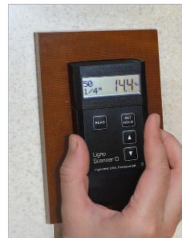
**Step 3:** Lignomat offers an external calibration check block TS for all Lignomat pinless meters. The check block for pinless meters from Lignomat is a material plate which produces a defined reading, when the meter is lightly pressed against its surface.
