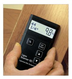
All Lignomat meters internally check and adjust the calibration. Manual recalibration is not needed.
