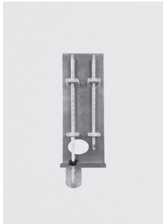
Dry-bulb-wet-bulb thermometers with measuring plate and wet sock bottle.
