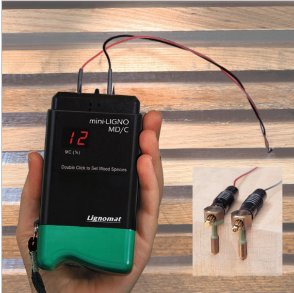
Mini-Ligno MD/C, and mini-Ligno DX/C with PK-mini Cables (up to 12' long) and PK Probes.
