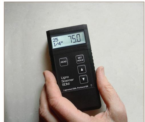
Building materials including concrete can be measured with one of the reference scales available in the Ligno-Scanner SDM. See ASTM F2659.
