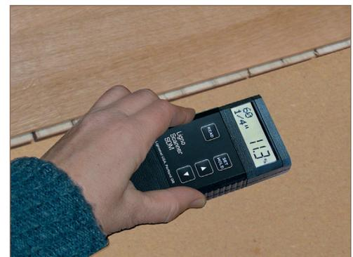
A favorite meter for floor applications with correction settings for domestic and tropical wood species, bamboo and subfloors. Can be self-calibrated for engineered products.
