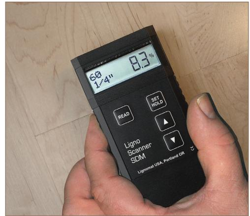
Lignomat's dual-depth scan meters have become the go-to meter in the flooring industry.
