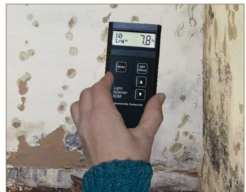
The Ligno-Scanner SDM is the perfect meter for the restoration specialist. In the photo, the SDM is used to check what needs to be removed in a moldy shower.
