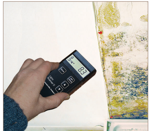
Lignomat's Scanner D can also quickly scan walls and ceilings to find areas of high moisture accumulations. However, if you need moisture percentages in wood, Ligno-Scanner D gives accurate moisture percentages.
