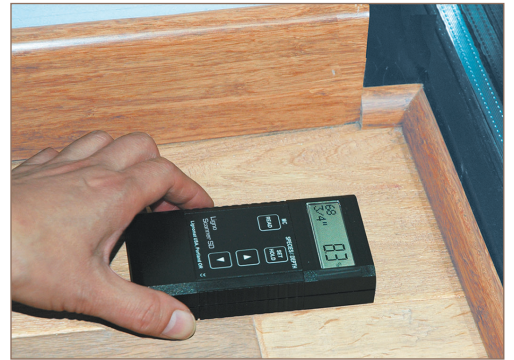
Once a job is finished, the meter can be used to take measurements to establish the present condition of the floor. For any problems later-on comparison to those earlier measurements can help to find the cause of any moisture related problems.
