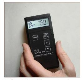
Building materials including concrete can be measured with one of the reference scales available in the Ligno-DuoTec BW.
