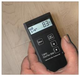
Lignomat's dual-depth scan meters have become the go-to meter in the flooring industry.
