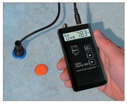
All accessories for in-situ probe testing of concrete are available form Lignomat, complying with ASTM F2170.
