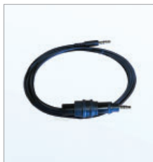
RH-CC cable for in-situ concrete testing with sleeve-seal to measure RH probes inside sleeves.
