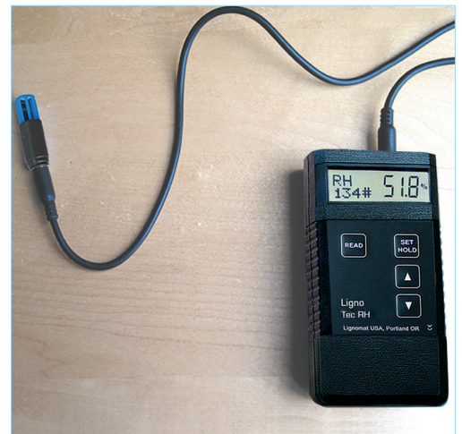
Cable extension to measure relative humidity in hard to reach, remote places (shown with Ligno-Tec RH).
