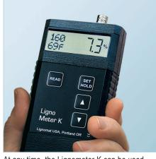
At any time, the Lignometer K can be used with the electrode E12 for spot-checking moisture conditions.
