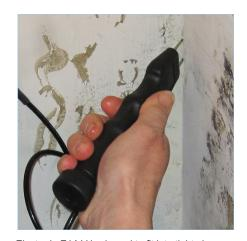
Electrode E14-V is shaped to fit into tight places where moisture is hidding but hard to measure.
