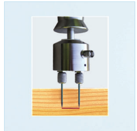
Teflon coated pins measure only at the tip. The E12 is the only tool to measure moisture at a defined depth.
