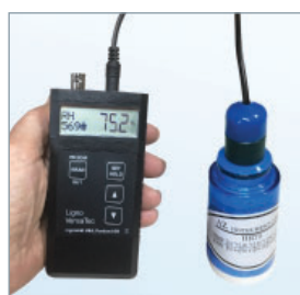
6. Salt Solution 75% Test
