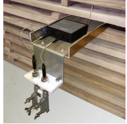
EMC measuring station with transmitter sends EMC measurements directly to receiver to keep track of ambient conditions and climate in a dry kiln.
