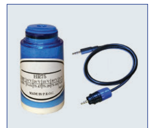
Salt solution to check RH BluePeg probes, RH 75%.
