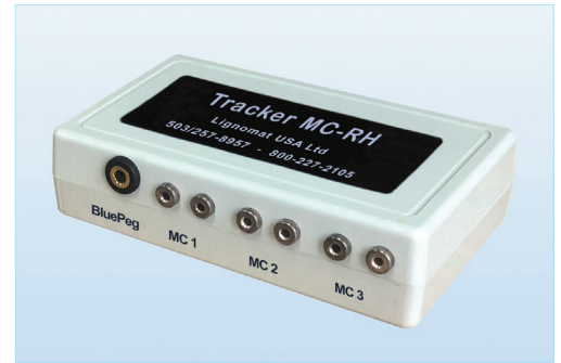
Tracker contains measuring circuitry for RH and MC: Front shows plug-ins for 3 moisture measuring cables and 1 RH cable.
