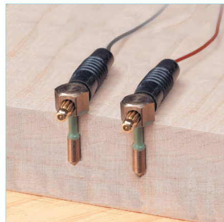
The probes have teflon-coated shanks, which insure that the moisture is measured at the depth the probes reach.
