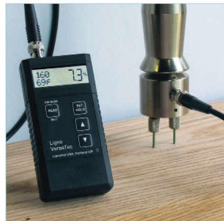
Slide-hammer to pin-point moisture distribution from surface to core up to 2" deep with DB pins.
