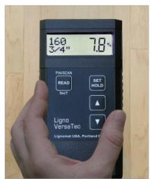
different depth levels in the same location, without moving the meter. This is the best way to compare surface and core moisture with the pinless measuring technology. Use the Ligno-VersaTec with a pin electrode to measure a moisture gradient in thicker wood.
