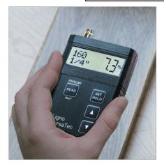
(1) Settings for the most common wood species, engineered products and building materials are listed in the laminated pocket guide included with the meter.
