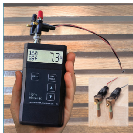
Place probes in the kiln, read moisture outside without opening a hot kiln. Multiple probes allow monitoring different areas in a kiln.
