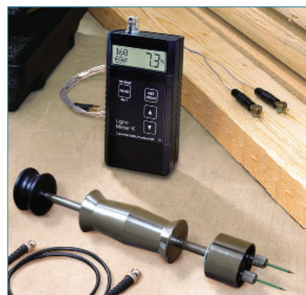
The K2-11M package includes the PK probe/cable system to monitor places that would otherwise be unreachable and the electrode E12 for measurements anywhere, anytime.
