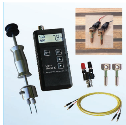
Lignometer K with extension cables and Electrode E12 for depth measurements.
