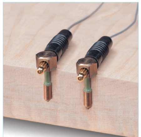
PK probes: Measure the core of the wood with teflonized probes.
