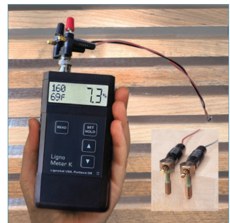
Place probes in the kiln, read moisture outside without opening a hot kiln. Multiple probes allow monitoring different areas in a kiln.
