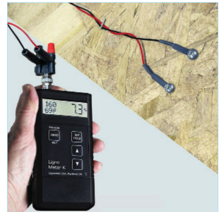
Install cables and pins in moisture critical areas. Measure periodically to check, if moisture problems are back.
