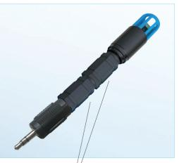
RH depth-adapters (#RH-DA) make RH probe longer to reach into crevices and behind walls. Also used when measuring concrete (ASTM F2170) for sleeves over 2.4" long.
