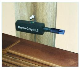
BL2 Memo-Chip with RH Thermo-Hygro probe used to monitor acclimation of a wood floor.
