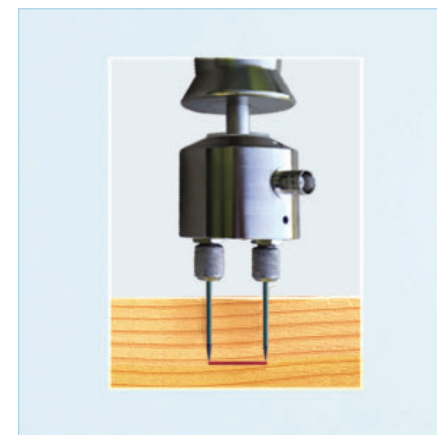
Teflon coated pins measure only at the tip. The E12 electrode is one tool to measure moisture at a defined depth.
