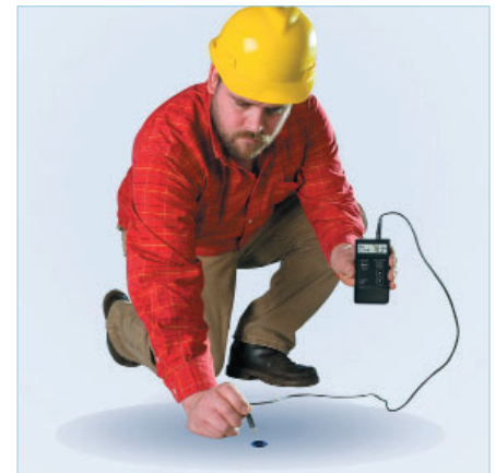
Lignomat's RH BluePeg system for in-situ RH concrete moisture testing, conforms to ASTM F2170 with reusable probes.
