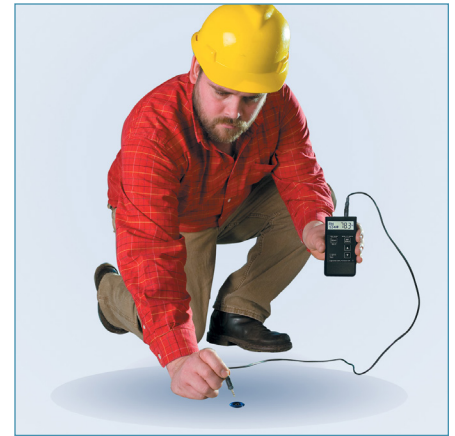
RH BluePeg Probe and sleeve used for in-situ concrete moisture testing.
