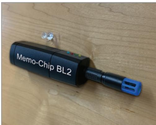
Connection between BL2 and RH BluePeg Probe via Adapter RH. Monitor for ambient conditions.
