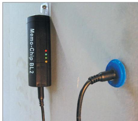
Connection between BL2 and BluePeg Sensor via RH Cable. Monitor for drying of insulation behind sheetrock wall.
