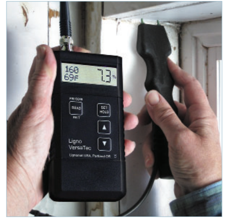
E14-V reaches easily into corners where the electrode E12 cannot be placed. Light-weight, sturdy and easy to use. Handle can be extended.
