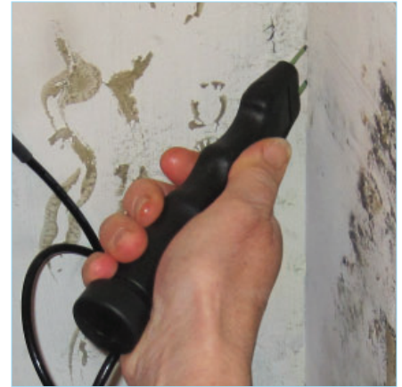
Inspector electrode E14-V fits in placed where other electrodes cannot measure
