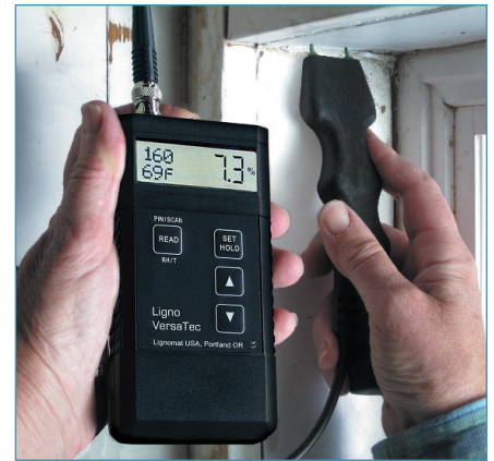
Pin electrode E14V measures in corners, around window sills, hard to reach places.
