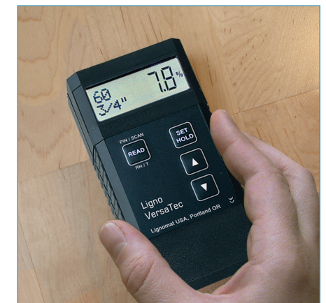
The Ligno-VersaTec is set up to take accurate moisture measurements in pin and pinless mode all species of wood and other materials such panel products, engineered floors and bamboo.
