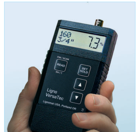
Ligno-VersaTec comes with a BNC connector for pin electrodes, a 35mm Stereo plug for RH measurements and 2 measuring plates on the back for pinless scan mode.
