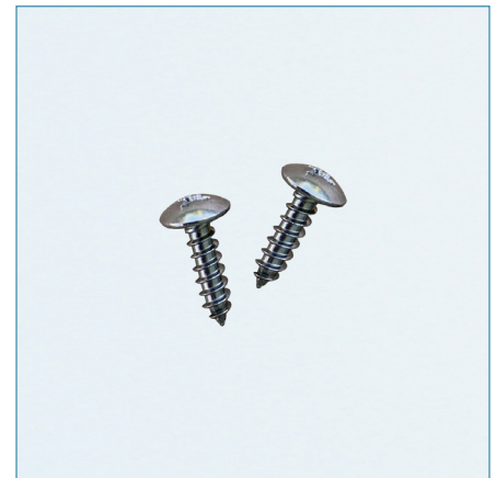
Stainless steel screws are used as probes for in-kiln monitoring
