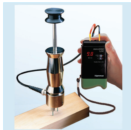
In-depth measurements detect unevenly dried wood and help avoid costly mistakes. Used when installing, inspecting floors and for restoration jobs.
