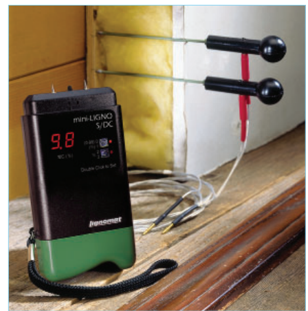
Hard-to-reach areas can be easily measured when adding the long EL pins. Reaching through insulation and wall boards.
