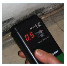
Mini-Ligno S/DC has a true percent scale for drywall, range 0-7.5%. Also included is a reference scale and a WME scale for drywall.
