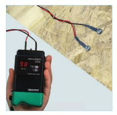
Install cables and pins in moisture critical areas. Measure periodically to check, if moisture problems are back.
