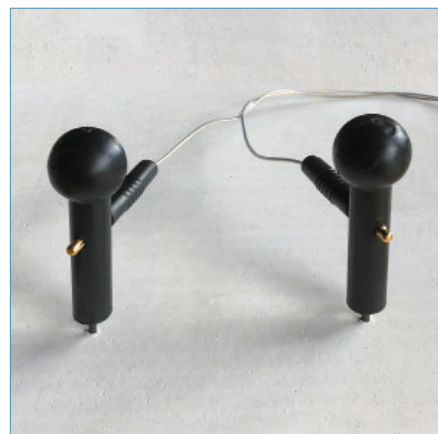
Electrode E16 allows wide distance between probes to allow for measuring cementitious materials incl. concrete.
