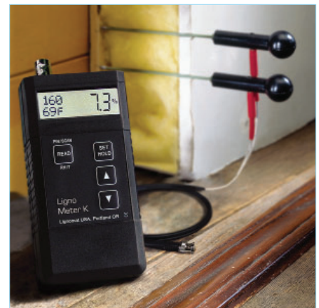
Hard-to-reach areas can be easily measured when adding the long EL pins. Reaching through insulation and wall boards.
