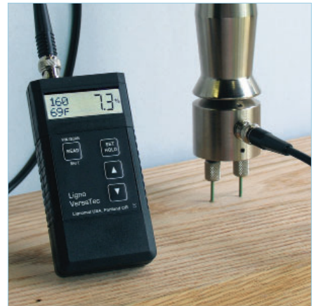
Slide-hammer to pin-point moisture distribution from surface to core up to 2" deep with DB pins.
