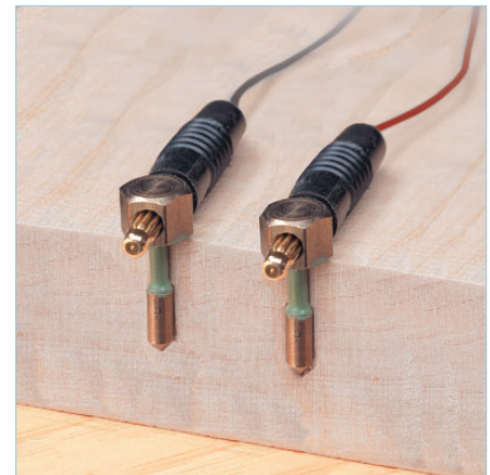
The probes have teflon-coated shanks, which insure that the moisture is measured at the depth the probes reach.
