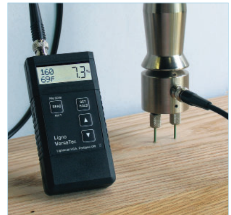
Slide-hammer to pin-point moisture distribution from surface to core.
