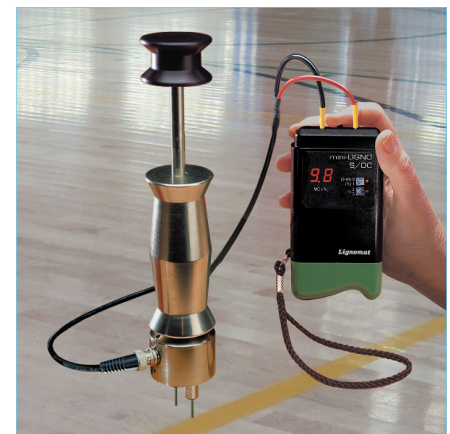
In-depth measurements allow measuring floor planks and sub floor without removing the floor planks. Used when installing, inspecting and repairing wood floors.
