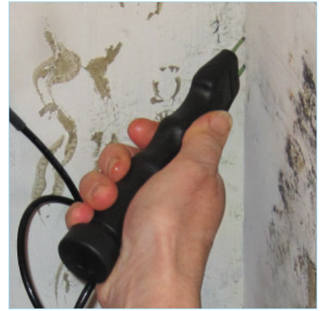
Inspector electrode E14-V measures in placed where other electrodes cannot reach, with EL pins up to 7" deep.
