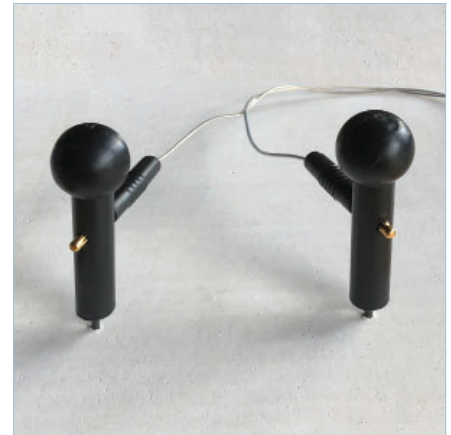
Measurements obtained from concrete or cementitious materials are not true percent values. They only can be used as reference numbers or comparative readings.
