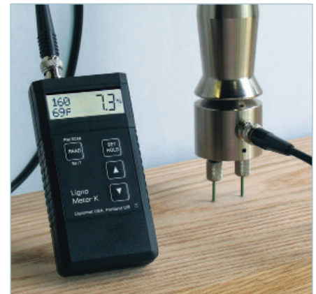
Slide-hammer to pin-point moisture distribution from surface to core. For quality control, for restoration jobs, when installing, inspecting floors.
