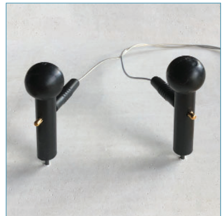
Electrode E16 allows wide distance between probes to allow for measuring cementitious materials incl. concrete.
