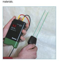
Adding the EL Pins allows reaching through insulation to measure structural components. EL Pins are 7" long, teflon-coated.
