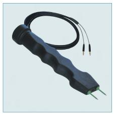
Inspector Electrode E14-m is designed to reach where moisture hides. E14-m is tough enough to hammer pins into hard
