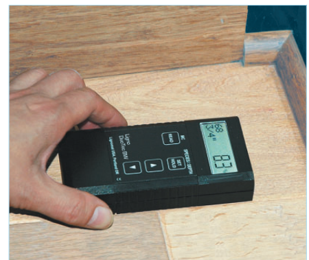
Multi-material, dual-depth pinless moisture meter: set for 1/4" and 3/4" deep to measure wood, bamboo, engineered panels, drywall, concrete,...
