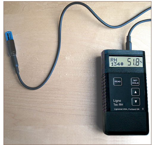
Cable extension to measure relative humidity in hard to reach, remote places.
