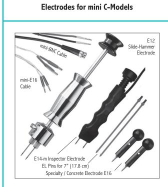
E12 Electrode is for measurements up to 2" (50mm) deep in wood and soft building materials (drywall, gypsum, plaster, etc.) Allows comparing surface and core moisture.
