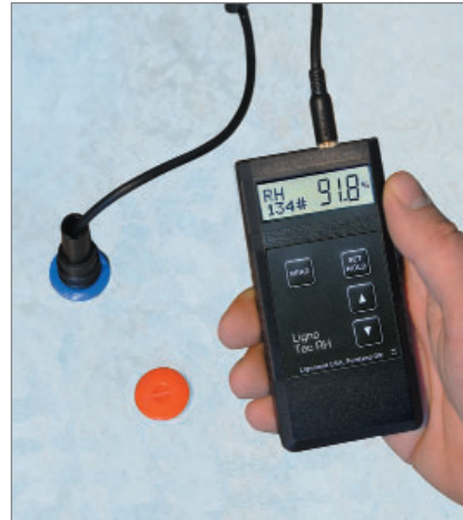
B In-situ concrete test with RH BluePeg probe and Ligno-Tec RH meter.
