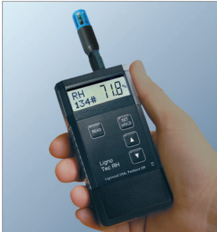
A Measurement of relative humidity, temperature and dewpoint, GPP of air.
