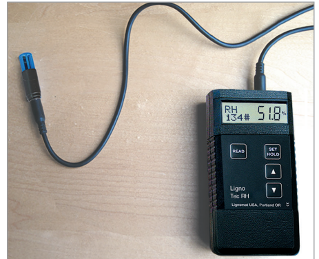
When the meter with RH adapter and probe does not reach far enough, use the RH cable for remote measurements.
