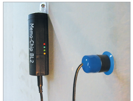
Monitor humidity changes with BL2 data logger. Measuring depth from 0.5" to 15". Opening is sealed with the RH-CB cable with sleeve-cover.
