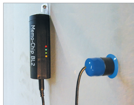
Monitor humidity changes with BL2 data logger. Measuring depth from 0.5" to 15". Opening is sealed with the RH-CB cable with sleeve-cover.
