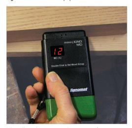
It is well worth to use a moisture meter for woodworking projects. Avoid cracked table tops, loose joints and failed glue lines.
